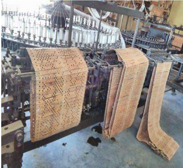
Figure 4. Lacemaking mechanism with punctured cards
