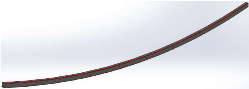
Fig. 3.5. Finite element model of test sample of top cord with location of heating zones
