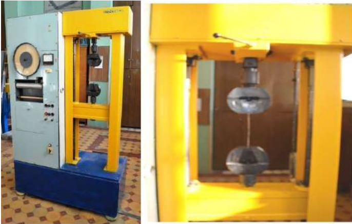
Fig. 3.21. Universal machine P-5 for static torsion testing
