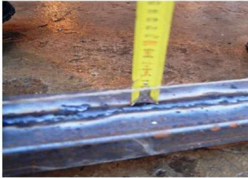
Fig. 3.9. Measurement of deflection at ends
