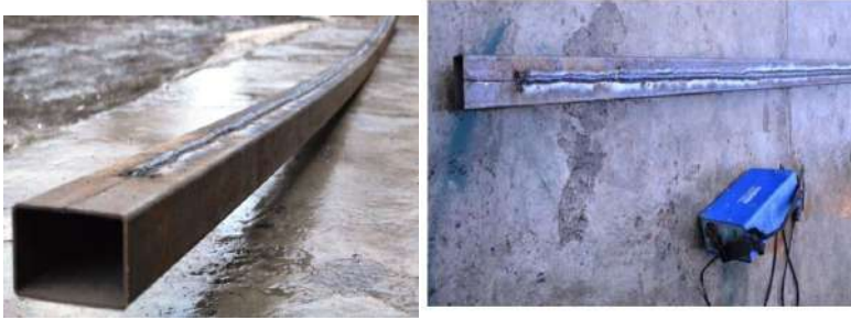
Fig. 3.2. Top cord test sample after technological welding
