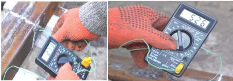
Fig. 3.13. Measurement of temperature under heating wedges
