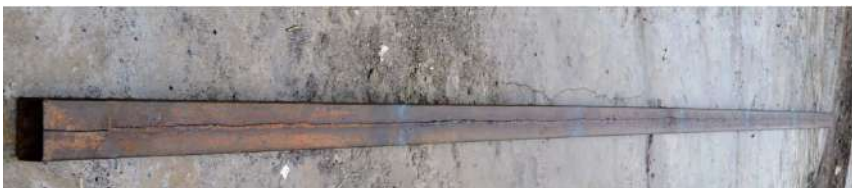
Fig. 3.14. Beam after thermal straightening
