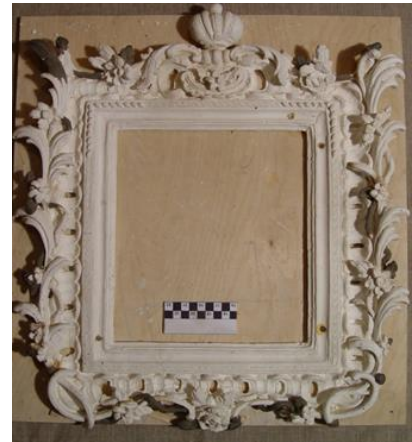
Figure 38. The transfer of the model from soft material to plaster to continue working in the authentic material of the monument – the wood of the linden tree
